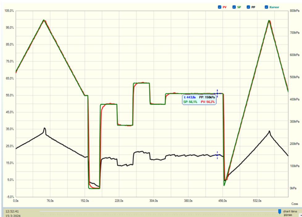
Fig.7 View of an exemplary time chart of the operation of a single-acting drive.
